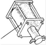
FOR MANUAL BOOST ONLY Spray WD-40 or equivalent into vent hole on bottom of boost unit
